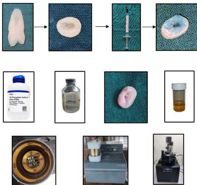
Figure 1: Sample preparation: Dental discs were prepared from extracted premolar teeth; discs were etched with 37% phosphoric acid; Discs were stored in phosphate buffered saline when not in use; dental discs were immersed or applied with respective agents; Gold sputter coating was done and examined under SEM.
